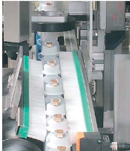
Infeed and cap inspection
